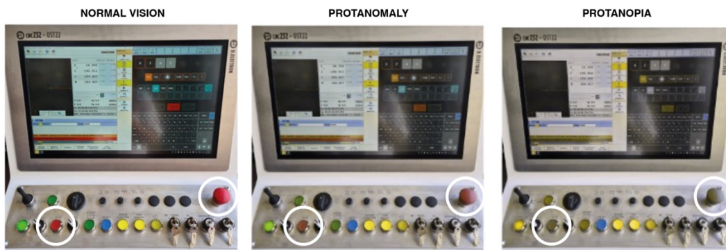
Fig.8 - Senergy Inail BRIC ID 40 project prototype under normal vision, protonomalous vision and protanopia vision
