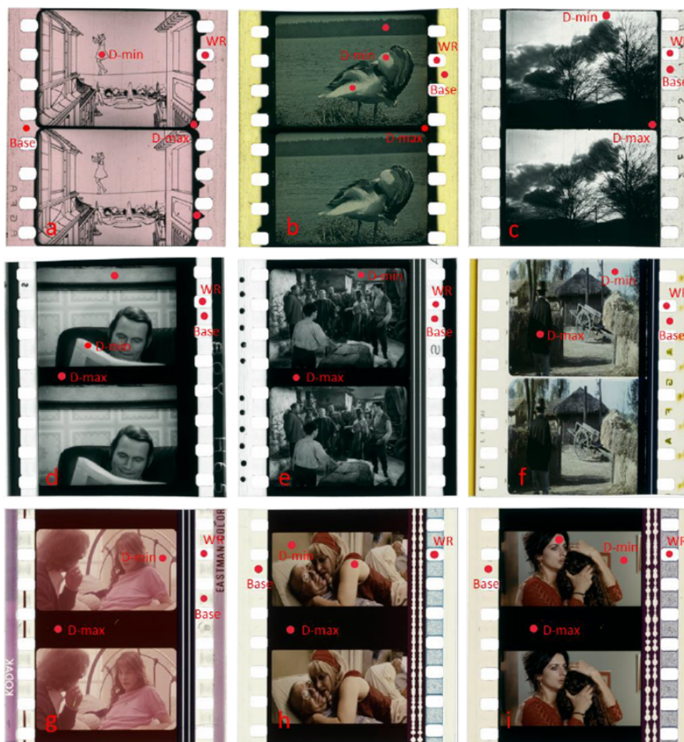
Fig. 13 - Color measurement points for film samples B1 (a) to B9 (i)
