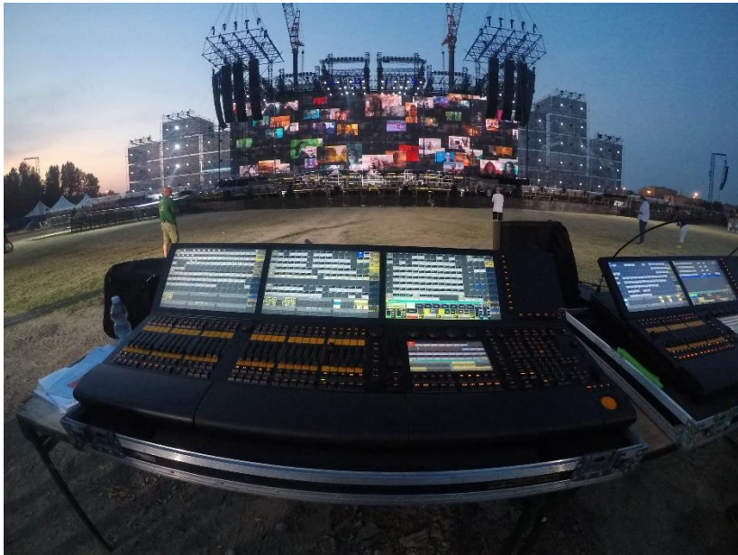
Figure 1. The presence of natural light (when working outdoors) and other light elements such as LED walls are parameters that must be taken into consideration when designing the lighting for a live show. Image courtesy: Giovanni Pinna.
