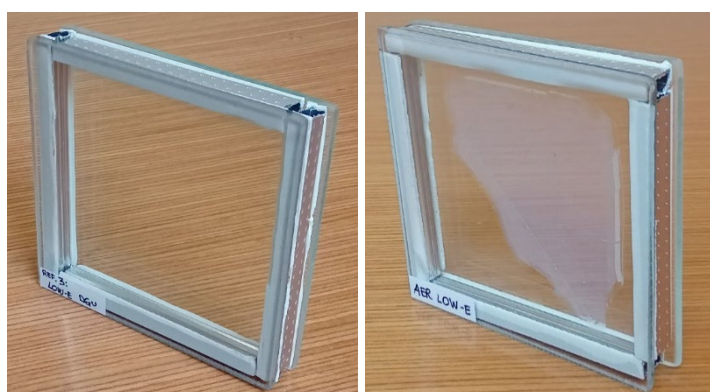
Figure 1 - Double glazing units prototypes: DGU low-e (left), DGU Aer low-e (right)
