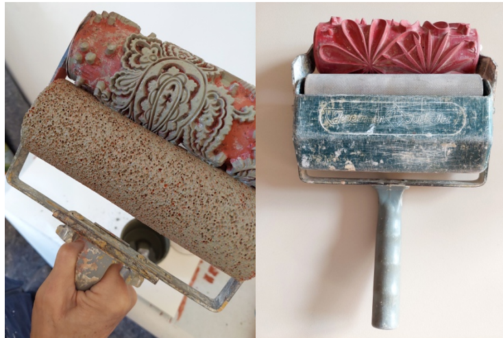
Fig. 4 – Pattern & foam feed roller within the roller frame
