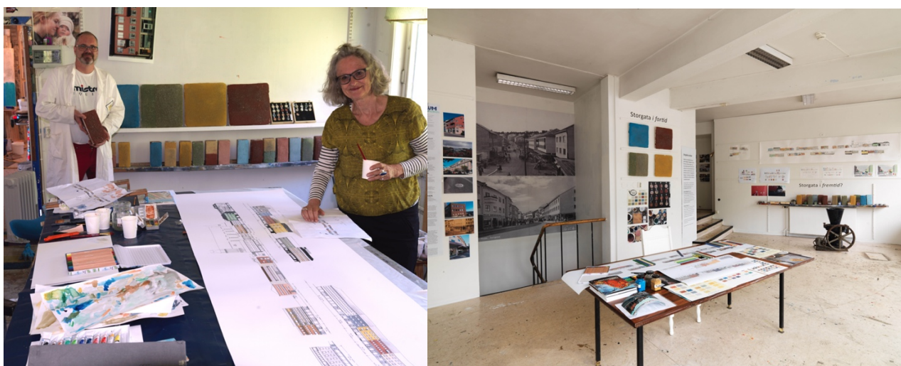
Fig. 2 Production of material samples for "Work in progress exhibition". Water colour renderings and lime based test plates from historic findings.
