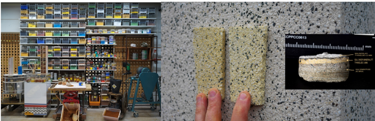
Fig. 4 Pilot project 1. Yellow Mineralite reproduction in Colour Lab. Test pieces made according to the core boron test from site and the macro photo. Background: Final result lacking the brilliant yellow ochre pigment.
