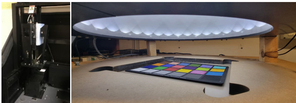
Figure 2 - Sample positioning inside the Solidspec-3700 for transmission measurements (left); Colorimetric characterization (right)
