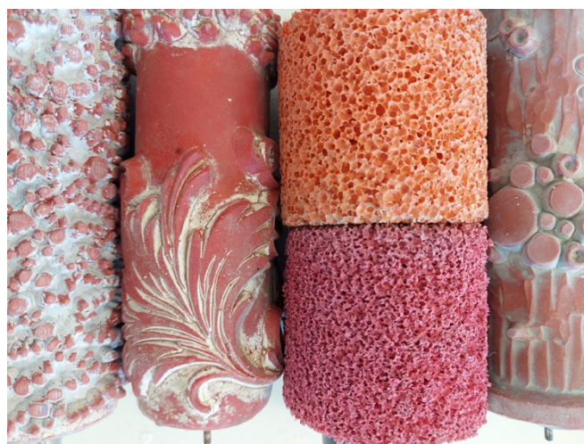
Fig. 6 – Pattern rollers and a two-color foam feed roller
