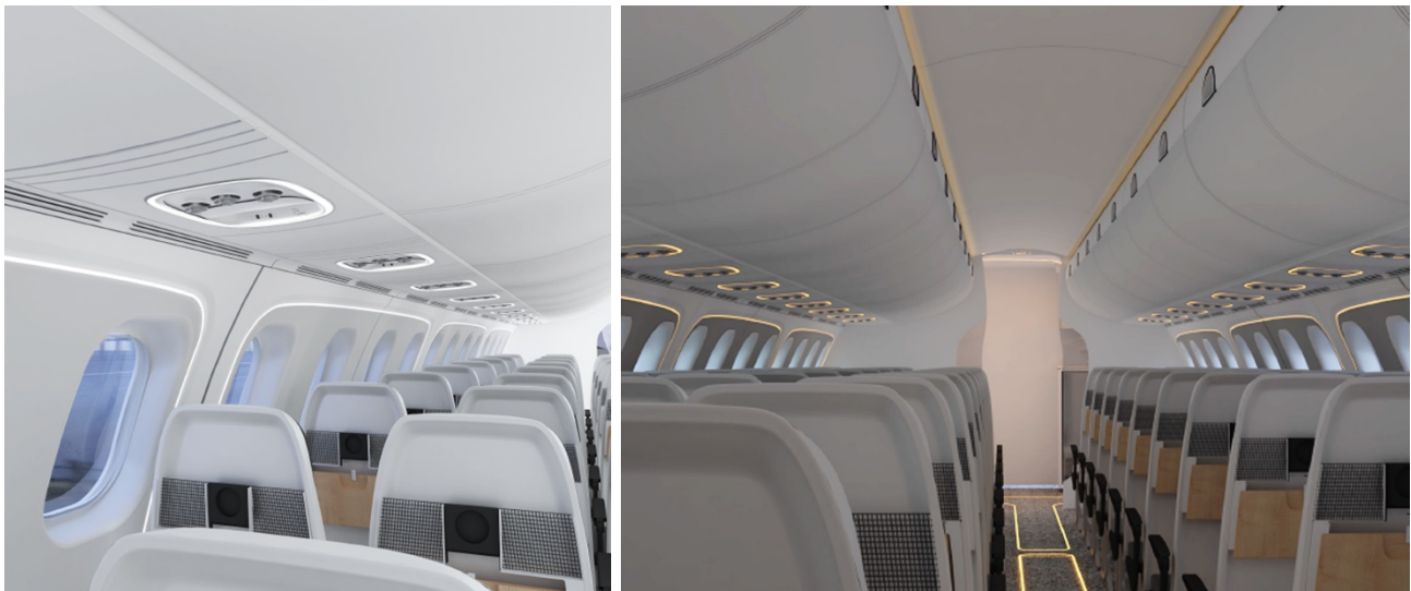
Fig. 7 – The preparation of the CASTLE cabin (concept design in collaboration with Pininfarina) with white light LEDs and possible variation of intensity and color through RGB LEDs.
