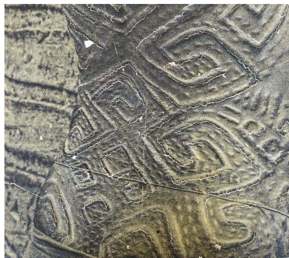
Fig. 13 – Detail of yellow discoloration on printed side of a Sammy Baloji inkjet print
