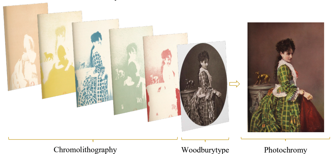
Fig. 4 – Diagram of a Photochromy print. Source: L. Vidal. Cours de Reproduction Industrielles (1882), adapted by the author.
