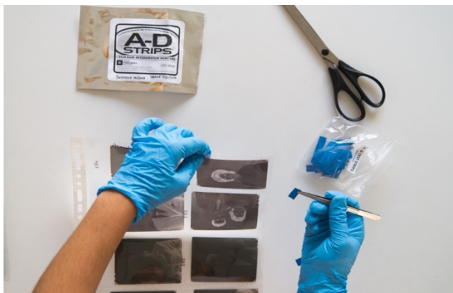
Fig. 2 Conducting the acidity test with the A-D strips.
