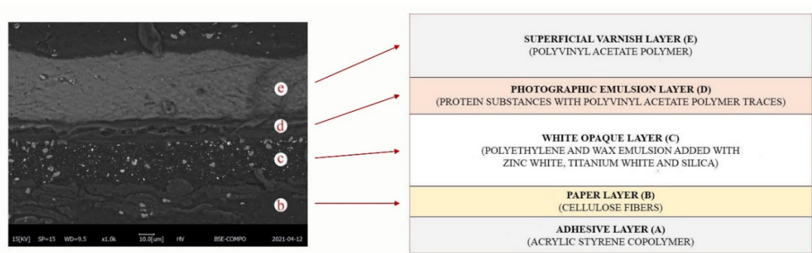
Fig. 2 Scanning electron microscope (SEM) image in which layers e, d, c, b can be identified (left) and graphical representation of the stratigraphic sequencing of the chromogenic print and surface layer. Layer a cannot be detected in the SEM image since the superficial layer was missing in the analyzed sample.
