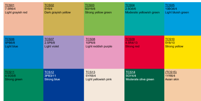
Figure 3: CIE test colour samples for use in CRI measurements (CIE, 1995)
