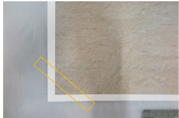
Fig. 10 – Area of yellow discolouration across one corner of the inkjet print where masking tape had sat above in the packaging
