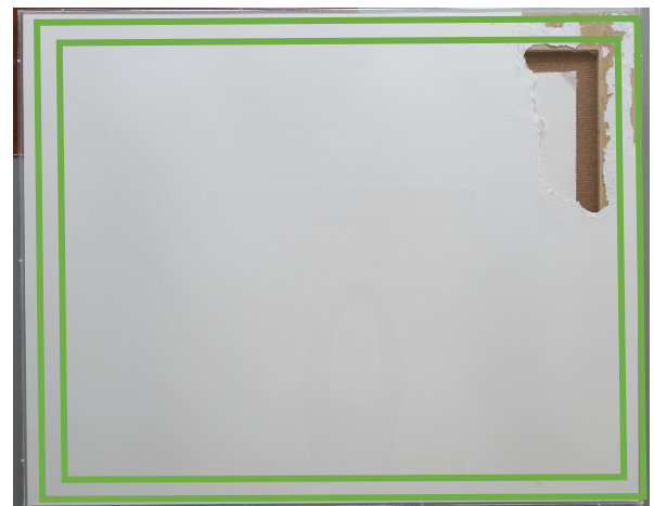
Fig. 6 – Green rectangles outline the area where the wooden subframe and adhesive film sat within the frame
