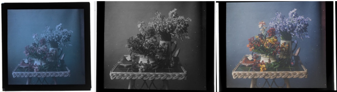
Fig. 8 - Unknown photographer, Paget lantern slide 8×8cm, ca 1921. Color calibrated scan (left), infrared scan (middle) and digital color reconstruction (right). Scanned at 4000PPI using DT Atom Rainbow MSI.
