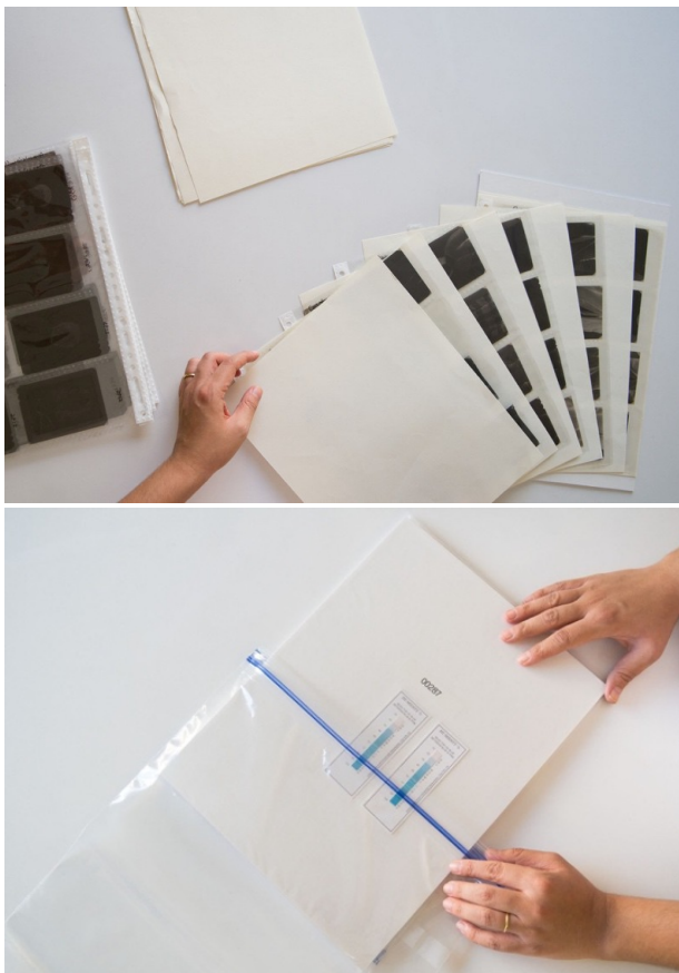
Fig. 7 Preparing films for cold storage by creating packages made from 4-ply mat boards, paper for buffering, humidity cards, and low-density polyethylene re-sealable bags.
