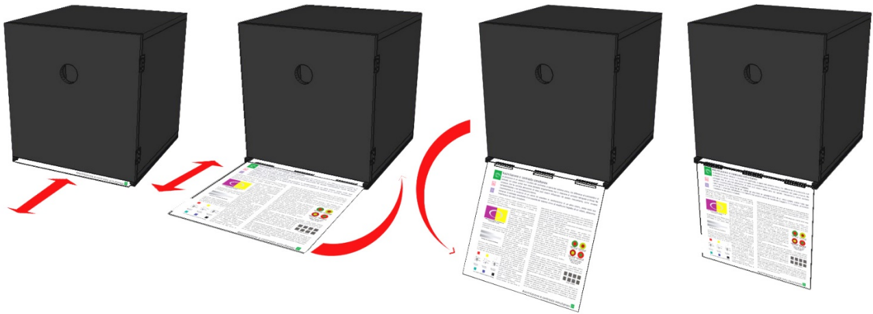
Fig. 2 – The black box design with the rails and the bounded info card.
