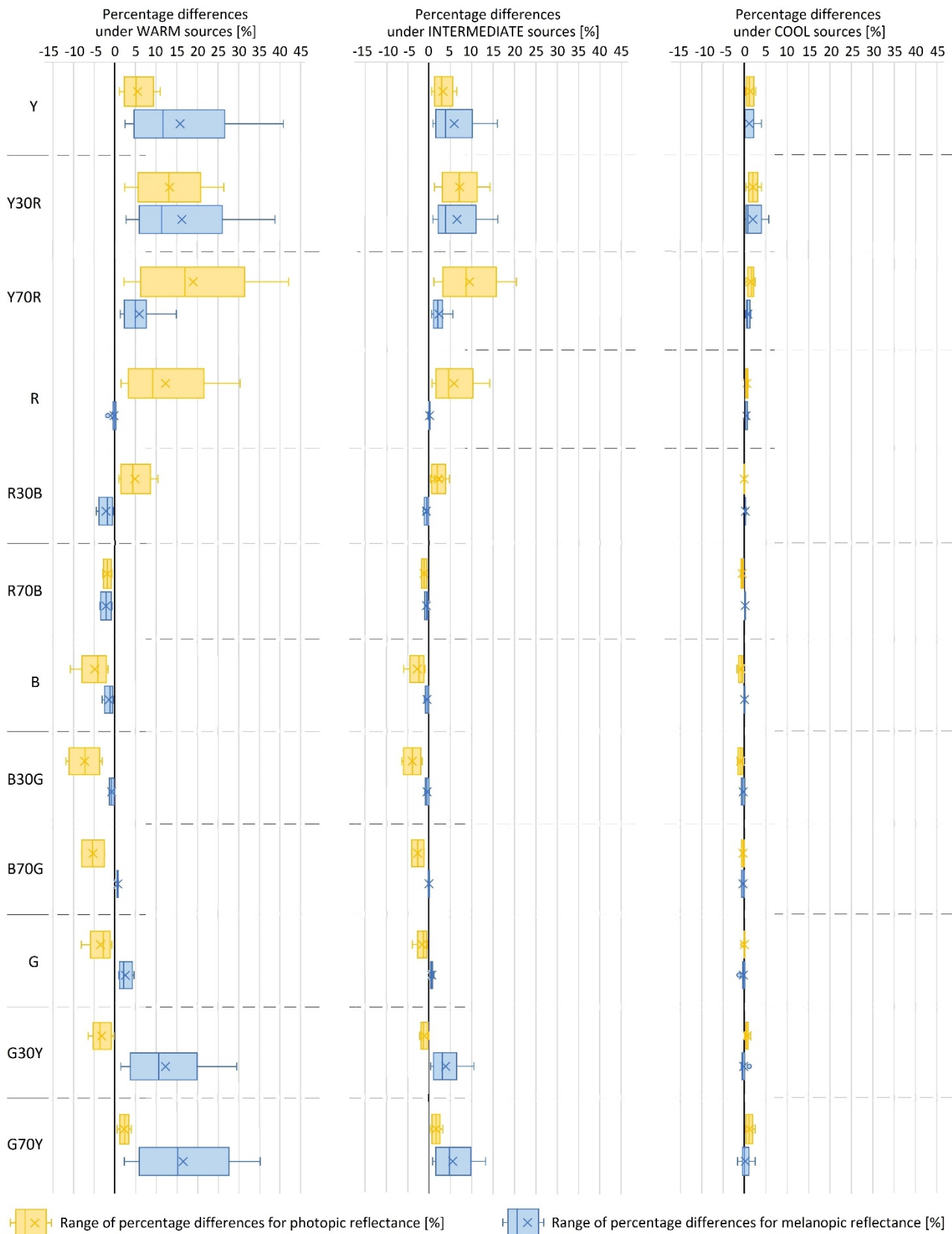
Fig. 4 – Variations in photopic reflectance (yellow) and melanopic reflectance (blue) under warm, intermediate, and cool LED sources.
