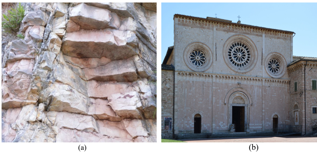
Fig. 4 - Assisi stone: a) aspect of the Scaglia Rossa formation and its use in religious buildings such as Saint Peter church in Assisi (b). (credits: E. Scopinaro).
