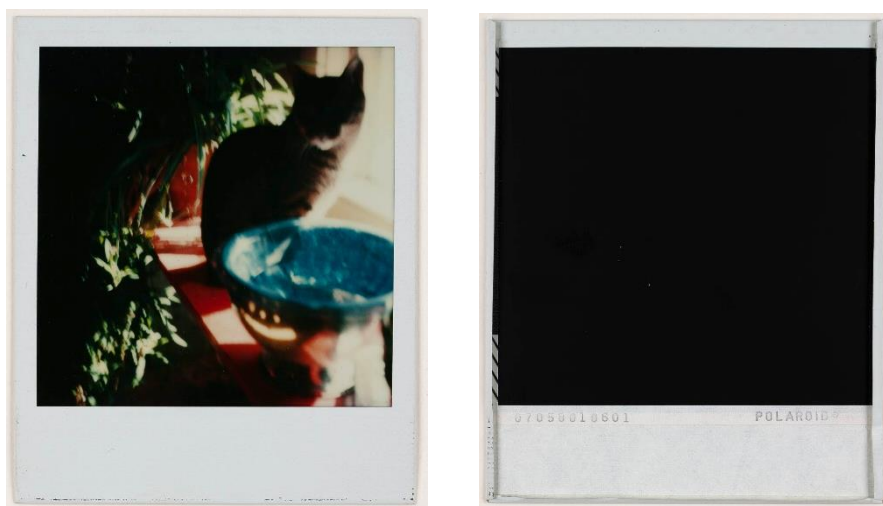
Figure 7 Front and back side of test material from Lot 2. On the left side one can see the square image area framed by the classic white foil around the edge. On the right side one can see the black polyester above the production code and the chemical pod.
