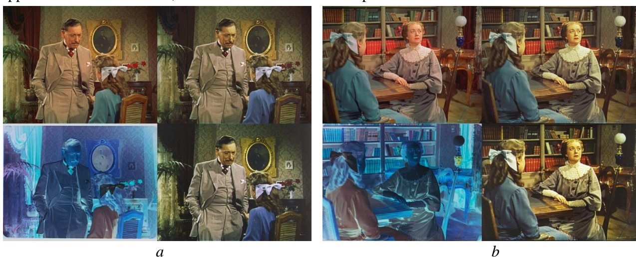
Fig. 2 – Two test cases of HEIDI UND PETER ( a and b ) – for each case, bottom left represents the input; top left is the result of the combined 1D LUT; top right is output after applying 3D LUT; bottom right is reference positive.
