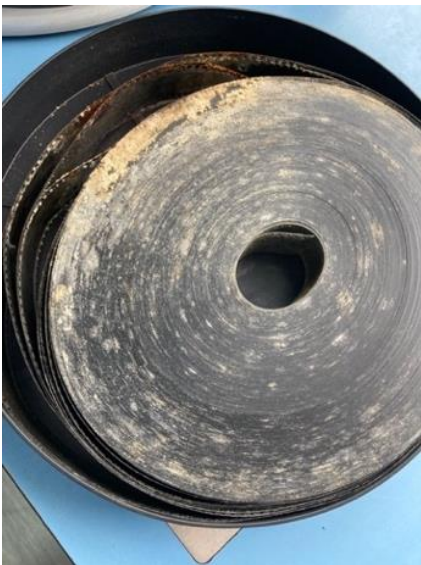
Fig. 3 - Condition of film deterioration
