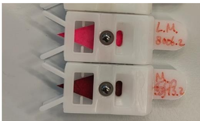
Fig 3 – Cut outs of Whatman filter paper to correct size and shape for PS-MS. The paper is loaded with ink from the cartridges, creating samples with only ink components present.
